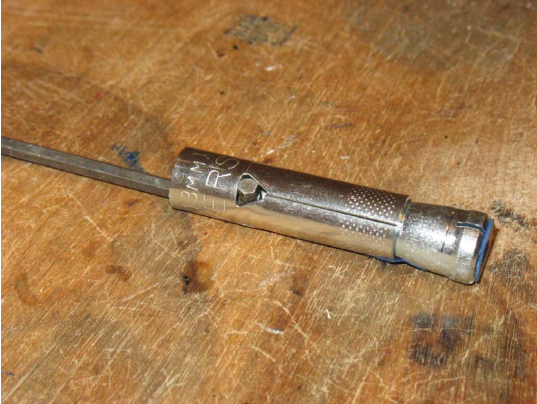
T-hex handle engaged into triangular hole of expansion sleeve
